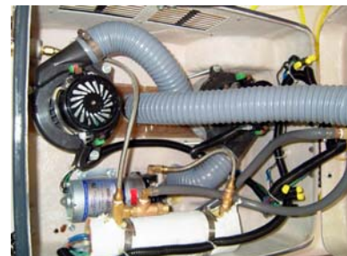
The Unit Has Easy Access to the Vacuum Motors and Pump Through a Suitcase Design
