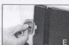
4. Pull the battery pack away from compartment.
